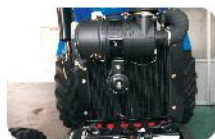
DRY TYPE AIR CLEANER WITH CLOGGING SENSOR
